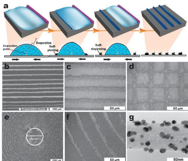
**Fig. 1** Illustration and results of the eDIP process. (a) The schematic diagram to show the eDIP process, (b) SEM image for line-type patterns of gold-CNT hybrid networks, (c) magnified SEM image for line-type patterns, (d) SEM image for grid-type patterns, (e) SEM image for circle-type patterns, (f) magnified SEM image for circle-type patterns, and (g) TEM image for a gold-CNT hybrid.
