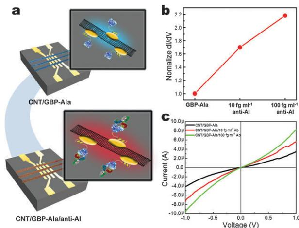
**Fig. 4** Electrical properties of the gold–CNT hybrid network by the GBP–Ala fusion protein and anti–Ala antibody interaction. (a) Illustration of the circuit preparation, (b) normalized  $dI/dV$  curve by the anti–AI binding, and (c)  $I$ – $V$  characteristic curves by the anti–AI binding.
