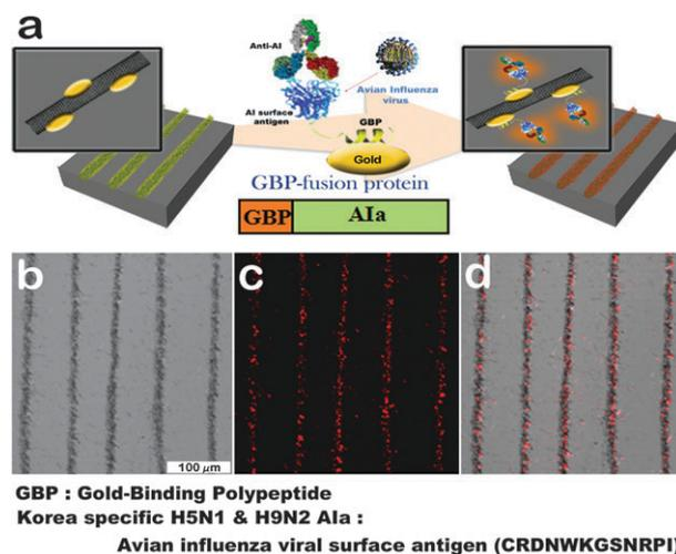
**Fig. 3** Illustration and results for the immobilization process for the GBP-AIa fusion protein onto the gold-CNT hybrid patterns. (a) Illustration of selective immobilization process, (b) optical image for CNT patterns after GBP-AIa immobilization, (c) fluorescence image after the sequential binding of GBP-AIa and Cy3-labeled anti-AI onto the gold-CNT hybrid line pattern, and (d) merged image of Fig. 3b and c.
