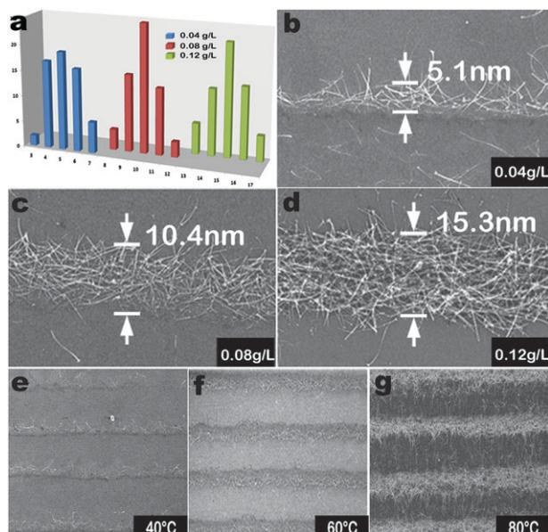
**Fig. 2** The effects of the stock solution concentration and evaporation rate. (a) The width distribution of gold-CNT hybrid patterns in different concentrations of the solution, (b)–(d) the SEM figures for patterned networks to show the width variation on the different concentrations of the stock solution, and (e)–(f) the SEM figures for network patterns to show the effect of the evaporation rate.
