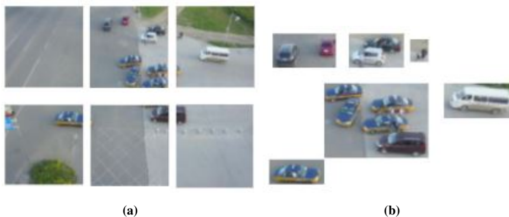
Figure 6. Visualization of (a) uniform cropping vs. (b) density crops achieved by our methodology. (a) corresponds to region proposals/ crops suggested by uniform cropping and (b) corresponds to cropped chips corresponding to MCNN with dilated convolutions. The uniform crops contain mostly background pixels. The crops made by density based methodology are more useful with respect to our task.
